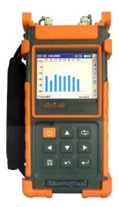
OCC-50 Handheld CWDM Optical Channel Checker is specially designed for CWDM installation, maintenance and troubleshooting, which allows you to measure and monitor power values of up to 18 CWDM channels. OCC-50 can replace high-cost Spectrometers and conduct quick and reliable measurements in all environments. Thanks to its light, compact and sturdy design, OCC-50 is the ideal tool for CWDM installation and maintenance technicians.
